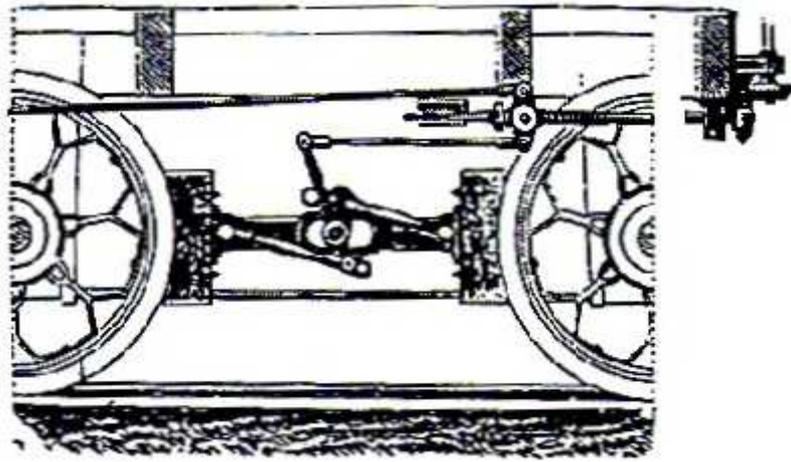
*Brake system controlled by screw and rods around 1837*
